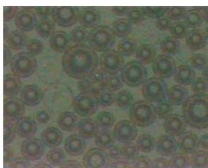
The coated hollow microspheres as seen in the picture on the left are buoyant enough to be used without a filter plate and the peptide synthesis described in this paper was actually performed in a separating funnel as seen below.
