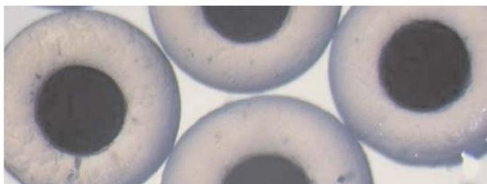
The standard commercially available seed beads are approximately 1mm diameter with a 0.4mm diameter hole and although standard jewellery beads have proved to be extremely effective we have also custom manufactured smaller glass cylinders which are 0.6mm length, 0.5mm diameter with a hole diameter of 0.4mm as in the following picture.
