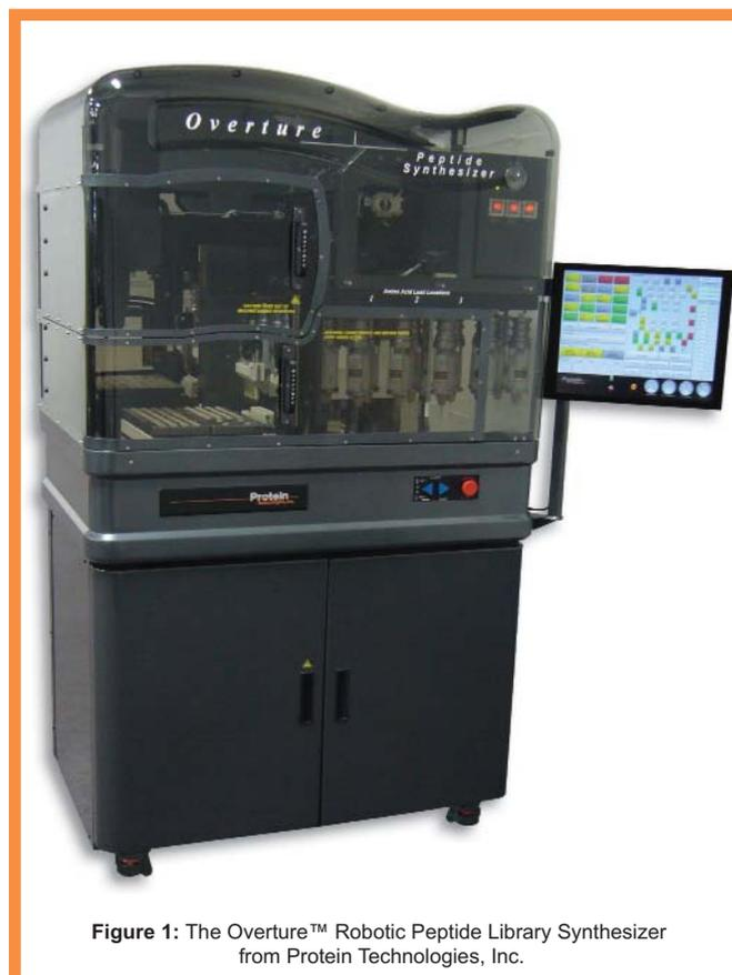
Figure 1: The Overture™ Robotic Peptide Library Synthesizer from Protein Technologies, Inc.
