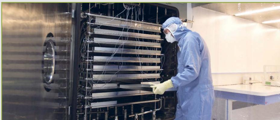
Large-capacity shelf freeze dryer for cGMP manufacturing
